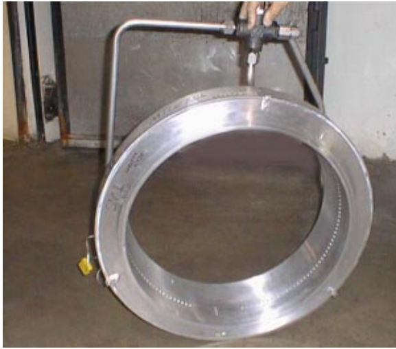
Fig. 5 Plenum airflow supply and distribution system
